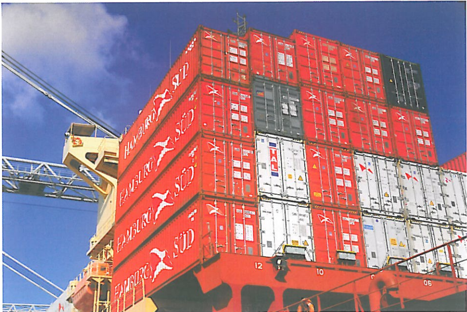
Container stack onboard with 40ft standard and 40ft high-cube containers
