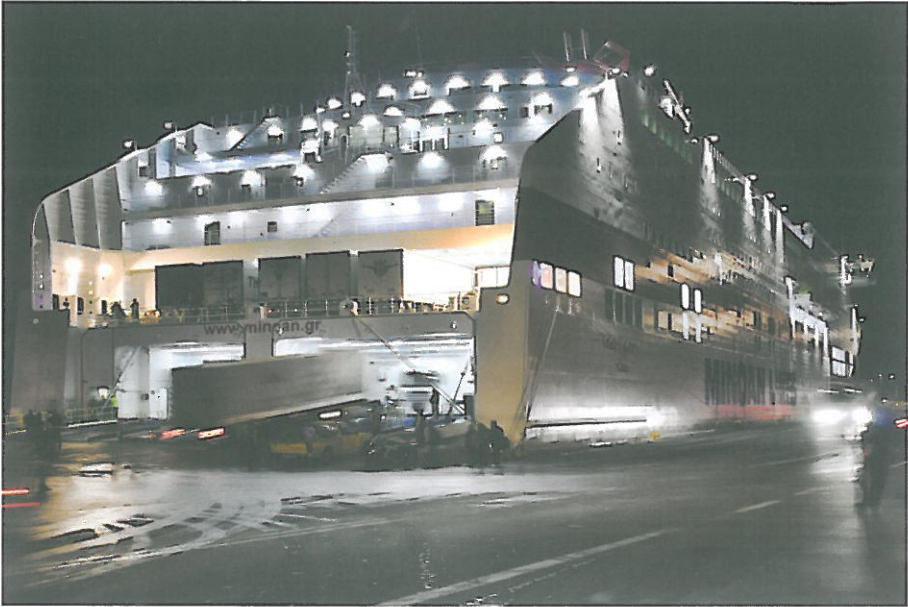
A typical freight ro-ro vessel loading via stern ramp
