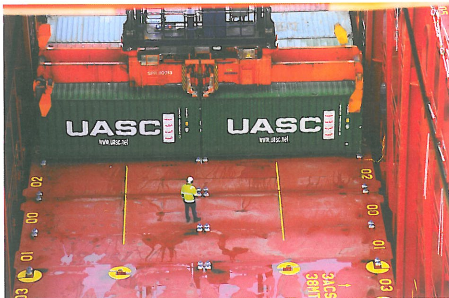
Row markings in a 20ft hold
