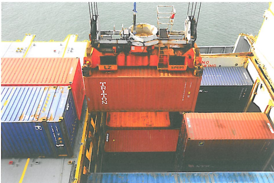
Each hold can take one 40-foot or two 20-foot containers
